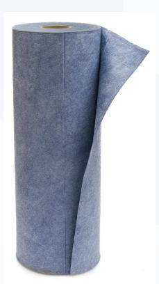
**DuraRug** is a needle-punched nonwoven geotextile made of 100% polypropylene staple fibers, which are formed into a random network for dimensional stability. Supplied in roll form, **DuraRug** resists ultraviolet deterioration, rotting, biological degradation, and naturally encountered basics and acids.
