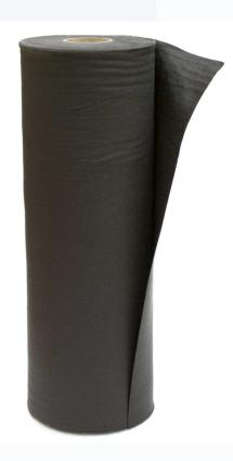
**DrillingMat** is a needle-punched nonwoven geotextile made of 100% polypropylene staple fibers, which are formed into a random network for dimensional stability. Supplied in roll form, **DrillingMat** resists ultraviolet deterioration, rotting, biological degradation, naturally encountered basics and acids.
